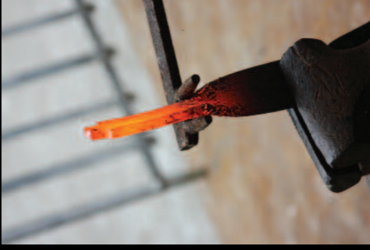
Twisting a wrought iron bar
