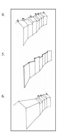
Building Lines and Building Heights Sketches 4 & 5 (Above): Note how the building lines meander and deflect. Note also how building heights tend to vary with a limited range. These are important principles of the Irish street-scape as reflected in Kilkenny's villages.
